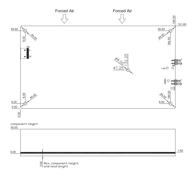
INPUT CONNECTOR (CN1): JWT A3963WV2-3P-D or EQU
