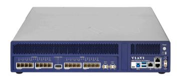
The Xgig 5P16 is a system platform that allows for simultaneous protocol analysis for PCle 5th generation protocol traffic at all layers of the stack. The exerciser capability supports compliance testing and advanced debug. It supports link speeds to 32 GT/s and widths up-to 16-lanes.
