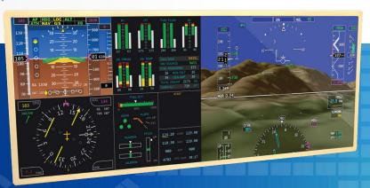
As the first dual-redundant large area display (LAD) of its kind, the LAD 2150 display head assembly (DHA) incorporates high-saturation color filters and 10-bit color depth affording a high-dynamic range of 1024 gray shades and capable of 1.3 billion colors.
