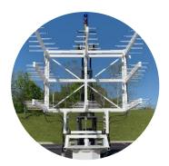
ARA's series of log-periodic antenna arrays supports a wide variety of applications requiring high-power transmission. These arrays are designed to meet strict beamwidth, gain, and power handling requirements. The log periodic design produces very broadband characteristics and a unidirectional radiation pattern. These antennas can be used to make accurate electric field strength measurements and individually calibrated antenna factor curve can be provided.
