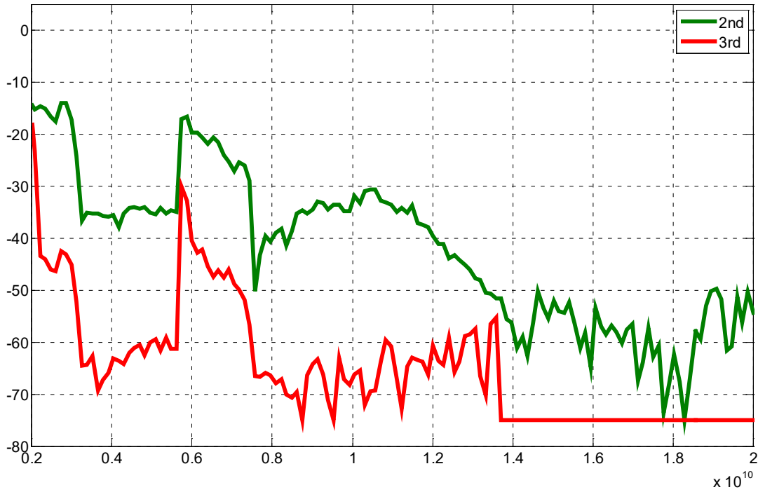
Harmonic output power [dBc] vs. frequency [Hz]
