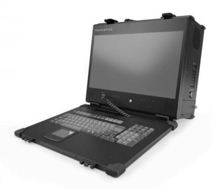
A battery-powered, compact, rugged portable with a 17.3" display and 4x expansion slots. Configurable with the latest Intel® Core™ or AMD processor.
