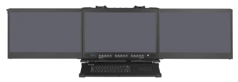
Triple 24" HD displays in a high performance, rugged portable setup. Designed as a flexible-use unit with 7x full-length expansion slots configurable for the most demanding applications.
