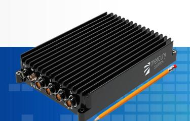
The NanoPAK™ i7 small form factor computer delivers performance and minimizes size, weight, power, and cooling (SWaP-C) for unmanned vehicle, ground vehicle, manwearable, and shipboard applications.
