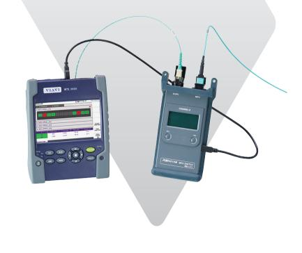
With the increasing amount of fiber being deployed into enterprise and datacenter networks, OTDRs are quickly becoming a critical part of enterprise test practices. Used to locate problems anywhere in the physical network, an OTDR is valuable for both certification and troubleshooting purposes.
